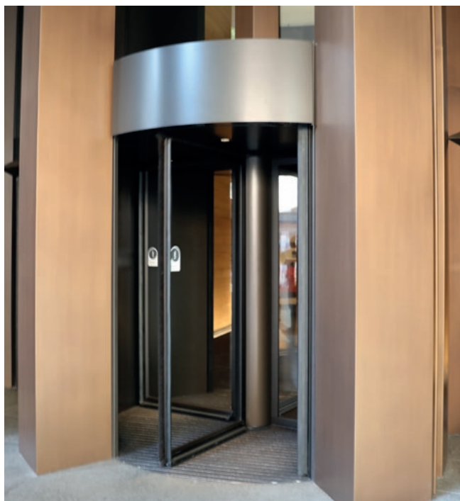
Figure 13: Four-leaf revolving door positioned with all segments open
